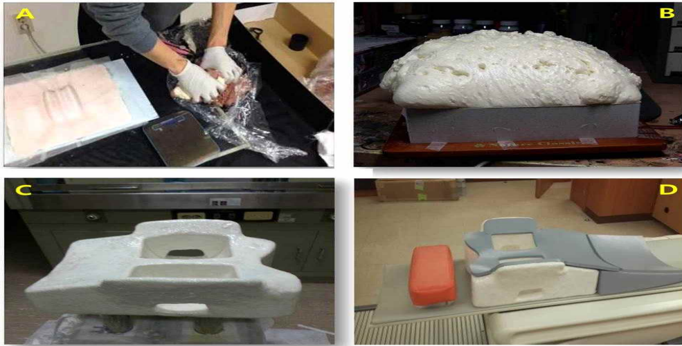
[Fig. 1] This is the process of making device. (A) The surface of the breast scan tool is wrapped. (B) this is preventive of flowing down urethane from a wooden box. (C) this is a breast scan tool removed from a mold. (D) FRP resin is attached to the surface of device.
