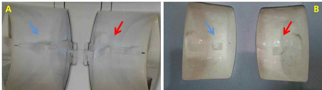
[Fig. 2] This show image that are MRI coil (A) and Breast tool (B) for measuring radioactivity counting rate. The plastic filled with 18F-FDG (0.5cc). Blue arrow is right side, red arrow is left side.
