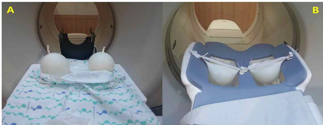
[Fig. 3] The balloons filled with water and 18 F-FDG were reproduced in supine and prone position on the breast tool.
