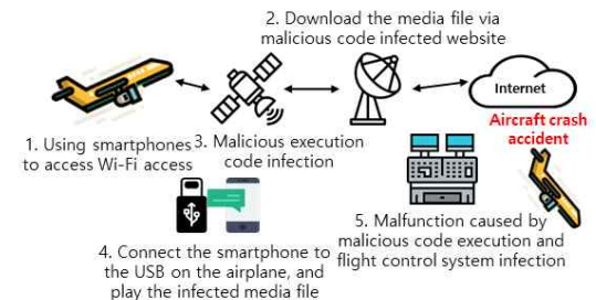
[Fig. 6] Harmful code infection and aircraft control system malfunction via in-flight Wi-Fi
