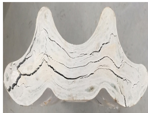
(b) Flexural geometry of wings-type GFRP clamping plate
