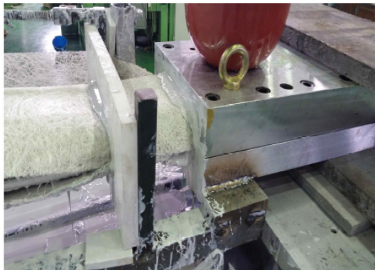
(c) Mold inlet supply after pre-forming
