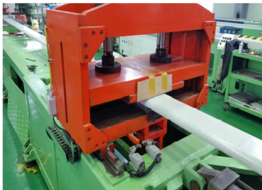
(e) Pulling device
