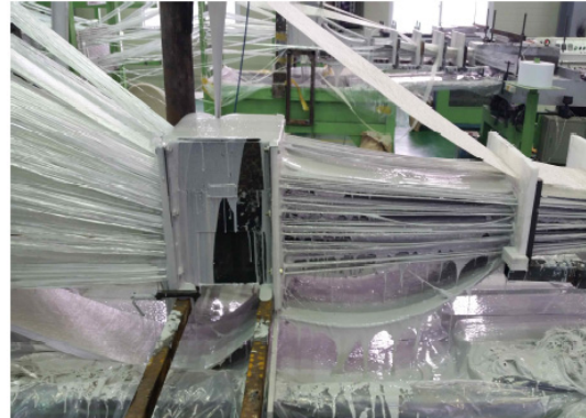
(b) Impregnation of vinyl ester resin
