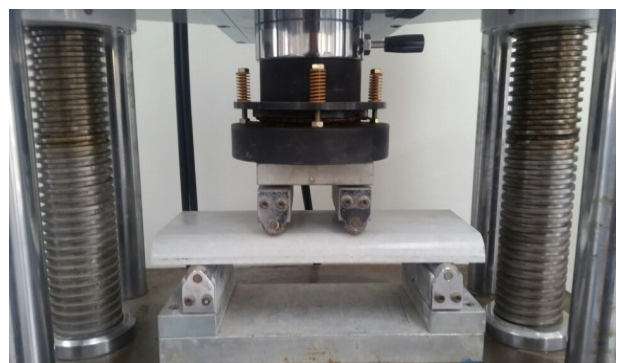
Fig. 3 Flexural load test set-up
