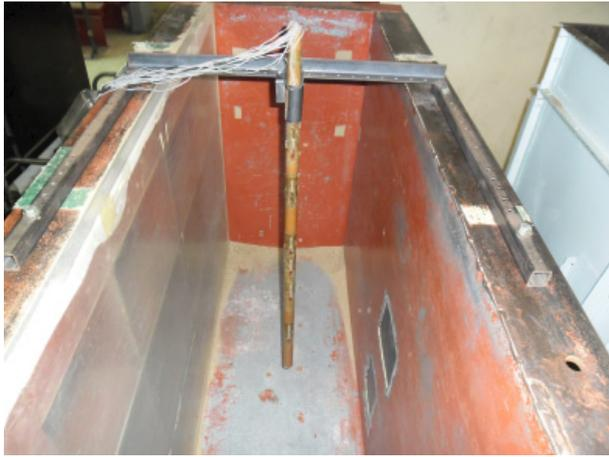
(a) Installing the model pile
