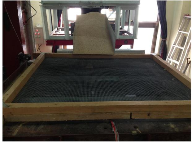
(b) Installing the #4 sieve and spraying the sand
