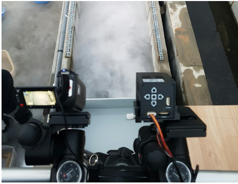
Fig. 11. Generation of fog condition with dry ice
