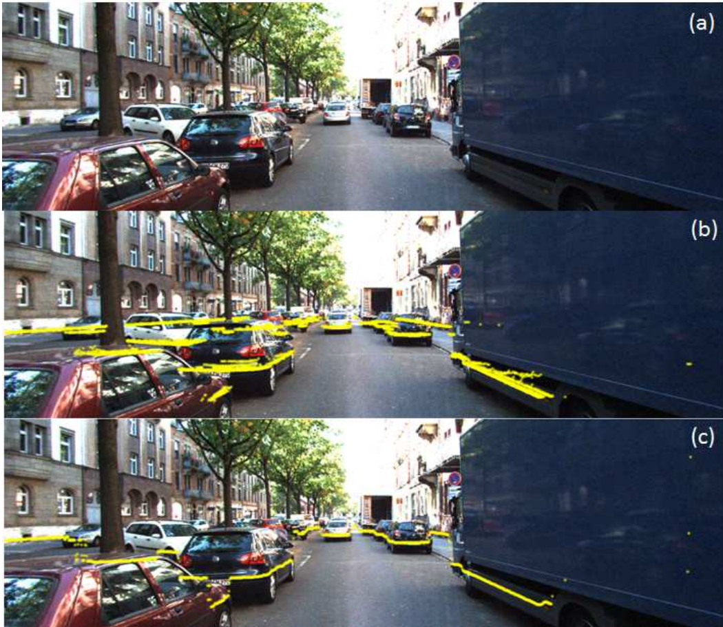
Fig. 2. (a) is the original input image, (b) is the projected image of the P_{plane} in the two-dimensional CCD space, and (c) is the result of generating the two-dimensional LiDAR Edge through filtering.
