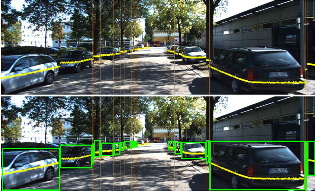
Fig. 4. A box proposal based on the boundary of a filtered 2D LiDAR Edge.
