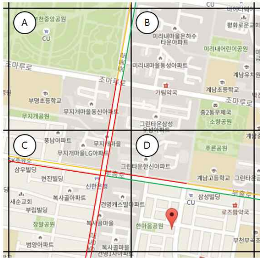
Fig. 3. Traffic data for each grid. In case of B, there is no road section included, so it is set to the same value as the road (road of A) at a close distance.
