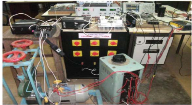
Fig. 4. Experimental setup of a 3 phase 2 level SVPWM controlled VSI.
