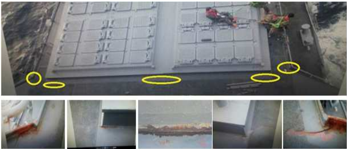
Figure 1. Status of KDX-II ○○ Ship Hull Crack
