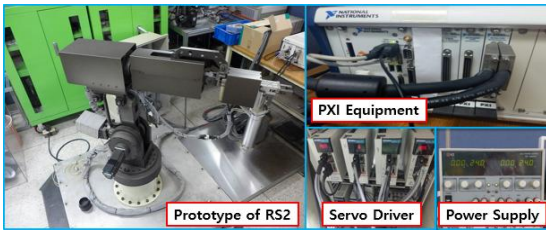
Fig. 1 RS2 system with servo driver and PXI® equipment
