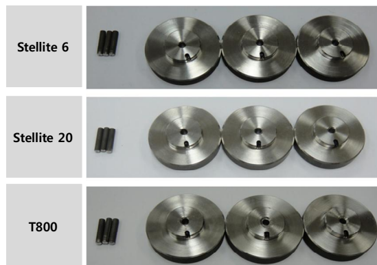
Fig. 2 Specimens for the wear test
