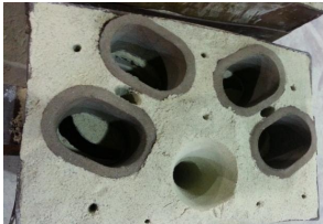
Fig. 16 Sand casting mold
