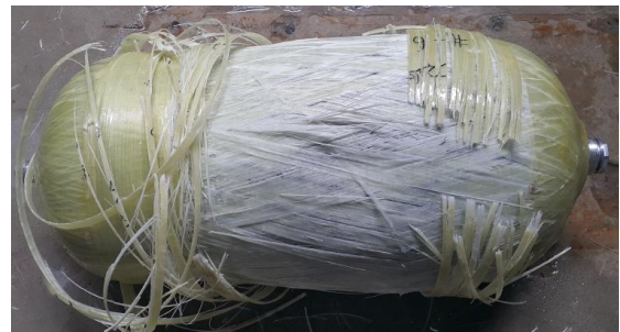
Fig. 10 Hybrid model after burst test
