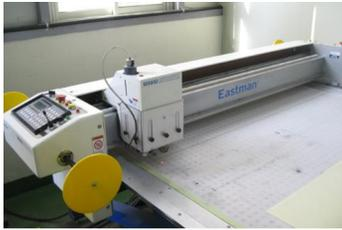
Fig. 7 Carbon fiber prepreg cutter
