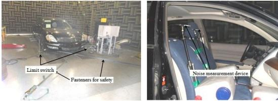
Fig. 15 Noise measurement device
