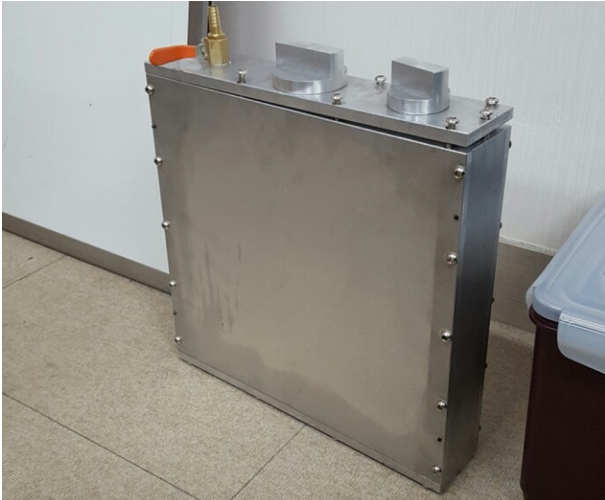
(a) Exterior of closed mold
