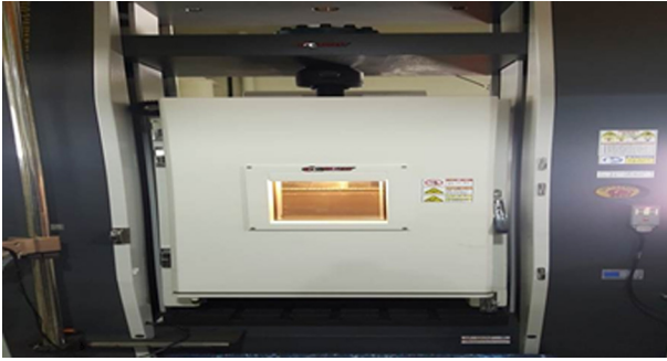
(a) Universal Testing Machine(UTM) under ultra-low temperature
