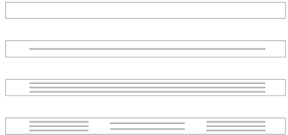
(a) Design model of Tie-plate : from upper initial model (None-Slot), 1-Slot, 3-Slots, 7-slots
