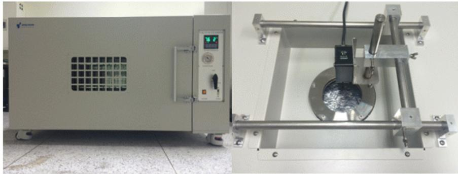
Fig. 6 Internal pressure measuring device for VIP
