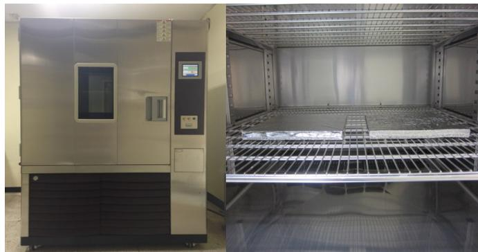
Fig. 4 Constant temperature and humidity chamber for aging test of vacuum insulation panels: exterior (left) and Interior (right)
