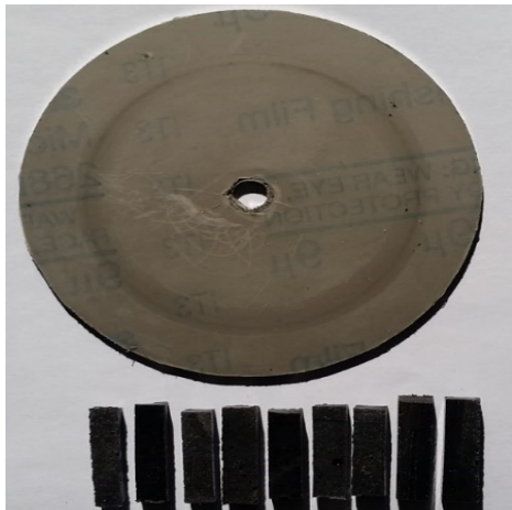
Fig. 2. Photograph of disc bonded SiC abrasive paper and wear specimens.
