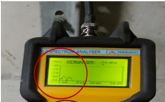
Fig. 10 Measurement result of communication signal from communication distance 500m on the underground utility tunnels
