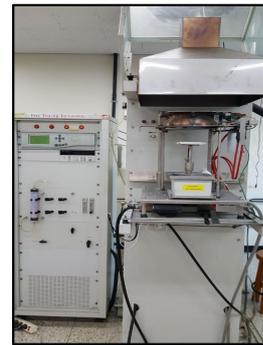
**Figure 3.** Dual cone calorimeter.
