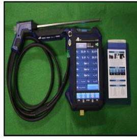
(b) combustion gas analyzer
