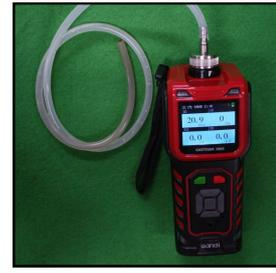
(c) H<sub>2</sub>S gas detector**Figure 2.** Experimental equipments.
