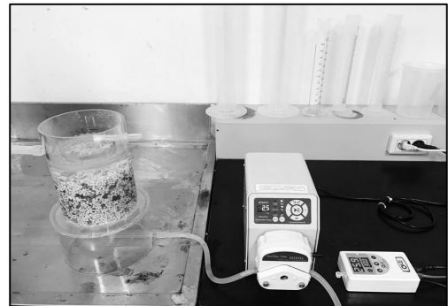
Fig. 1. Photograph of the lab-scale plant for the sulfur denitrification.
