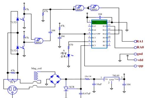
Fig. 8. Diagram of Serial Arc Detector
