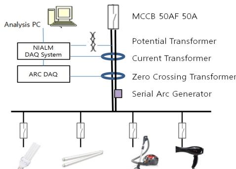
Fig. 4. System Structure
