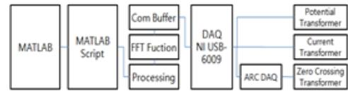
Fig. 5. Data Processing Structure
