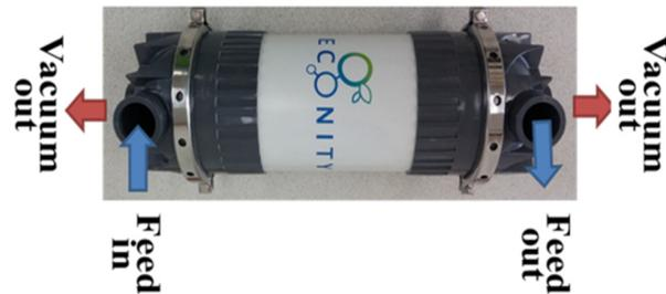
Fig. 3. The picture of the VMD module of Econity
