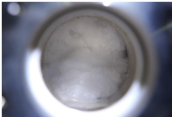
Fig. 8 Visualization of CO<sub>2</sub>-hydrate slurry in a reservoir tank.
