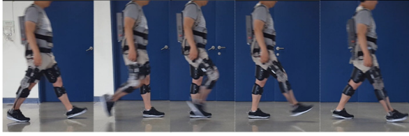
Fig. 9. Gait assistance experiment with EROWA
