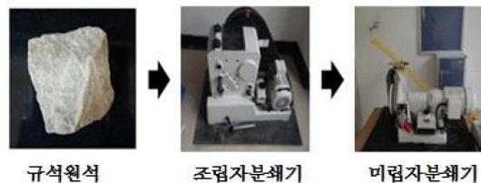
Fig. 2. Particle grinding process.
