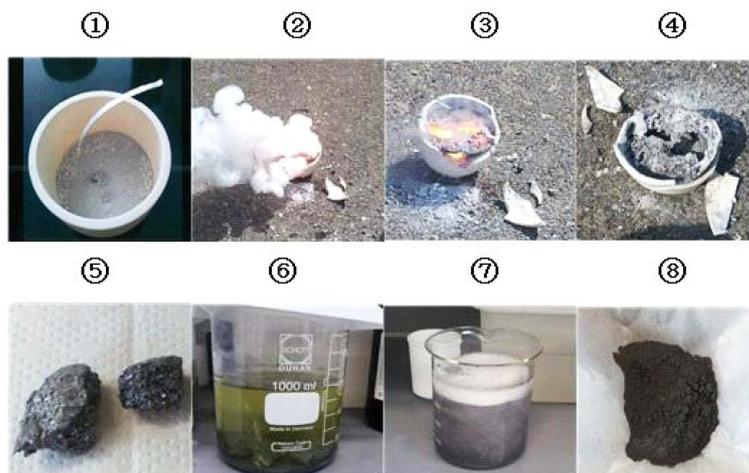
**Fig. 3.** Process of thermite reaction.
