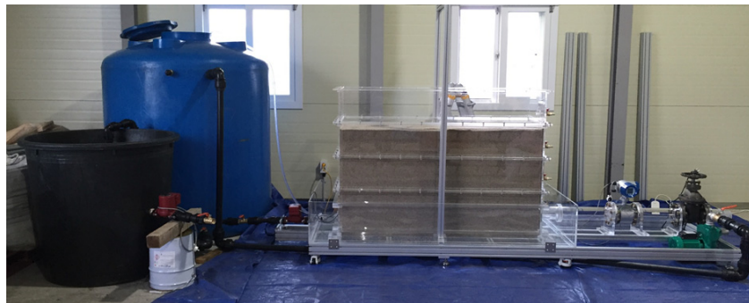
Fig. 1. Appearance of lab scale riverbed filtration experiment
