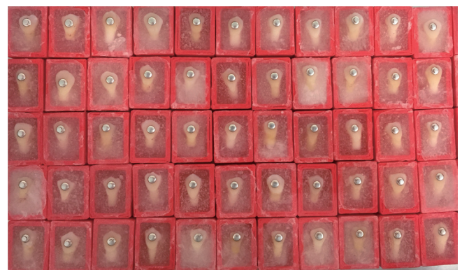
Fig. 3. Human premolar embedded in the mold with orthodontic rein.
