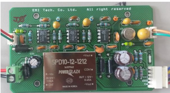
Fig. 8. PCB fabricated for signal processing
