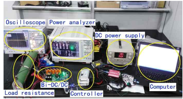
Fig.5. Efficiency test bench of the Bi-DC/DC
