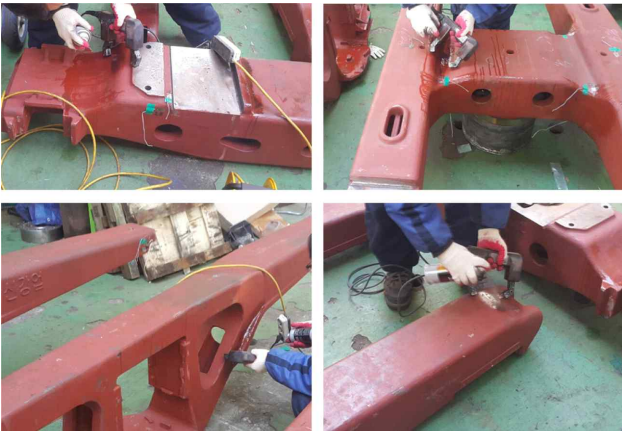
Fig. 7 Non-destructive evaluation after the static load test
