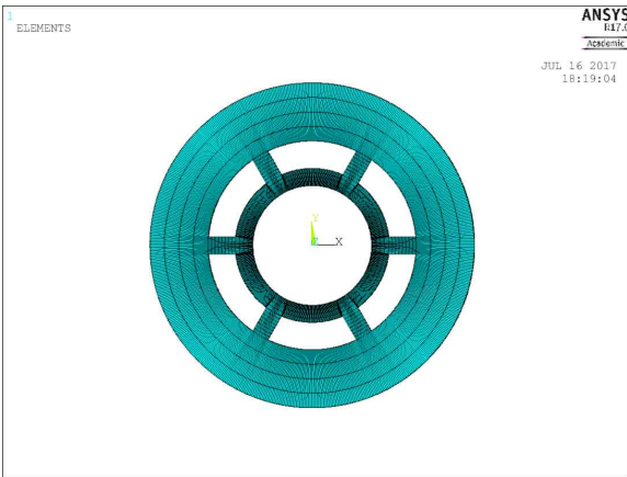
Fig. 3 FEM model of the wheel force/moment sensor
