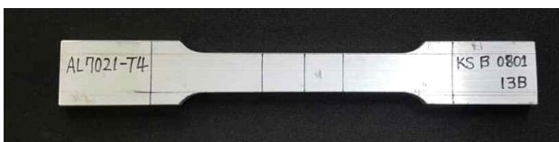
Fig. 1 Extension test specimen of KS B 0801 13B
