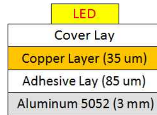
Fig. 6 Laminated layer structure of MPCB
