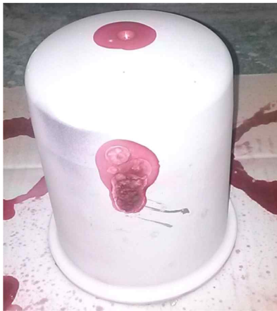
Fig. 19 Pinhole defects during penetrant inspection of sleeve parts
