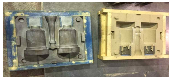
Fig. 17 Wooden pattern and casting mold for sleeve sand casting
