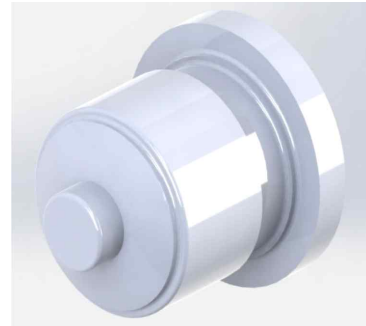
Fig. 4 Wooden pattern of sleeve sand casting
