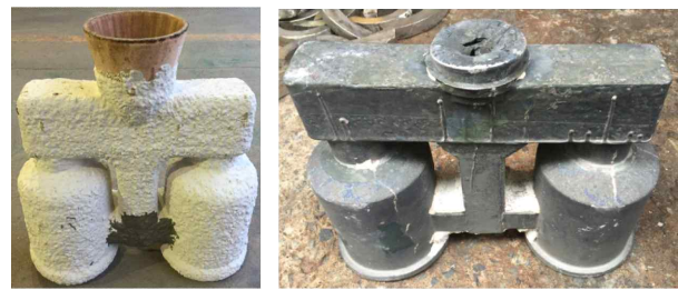
Fig. 15 Casting mold and cooling process for sleeve precision casting
