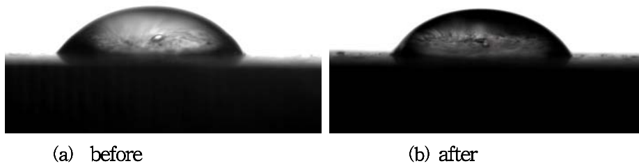
[Figure 8] Contact angle of specimen surface coated PVA before (a) and after (b) durability experiment.
