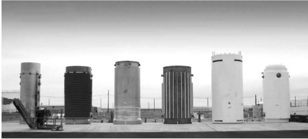
Fig. 3. Demonstration casks stored at INTEC of INL (NAC-I28, CASTOR V/21, REA 2023, MC-10, VSC-17, TN 24P from left) [13].
