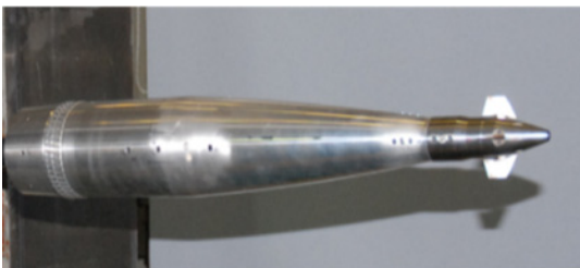
Fig. 7. Scaled-down model for the wind tunnel test
