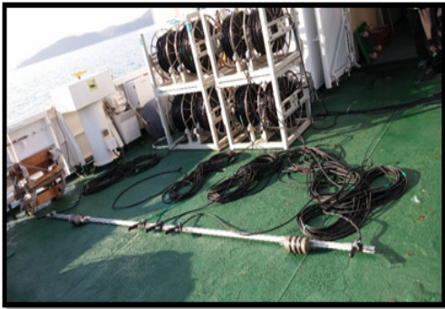
Fig. 5. Hydrophone arrangement for DF
