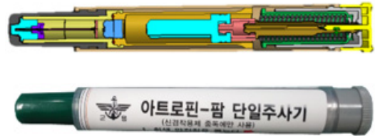
Fig. 3. Multi-chambered single autoinjector(2in1)
