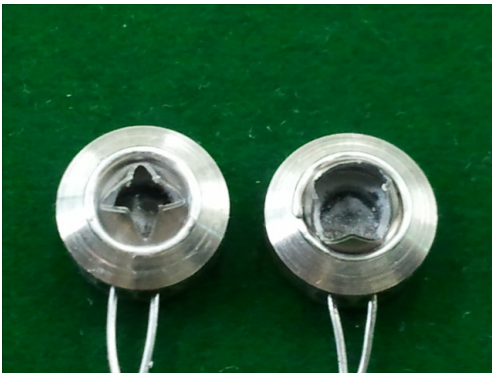
Fig. 6. Shape of the electronic igniter after firing
