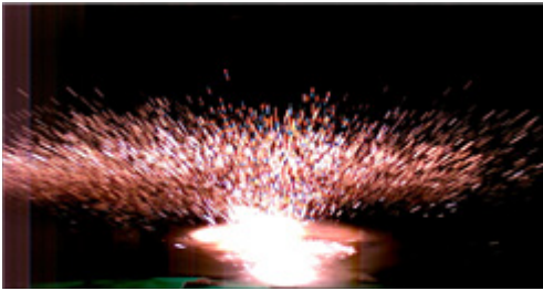
Fig. 5. Flame shape of the electric igniter
