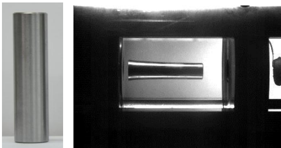
Fig. 11. Taylor impacting test specimen ( v = 183.3 \text{ m/s} )
