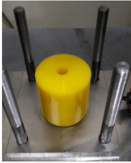
(a) A rubber spring installed on lower plate
