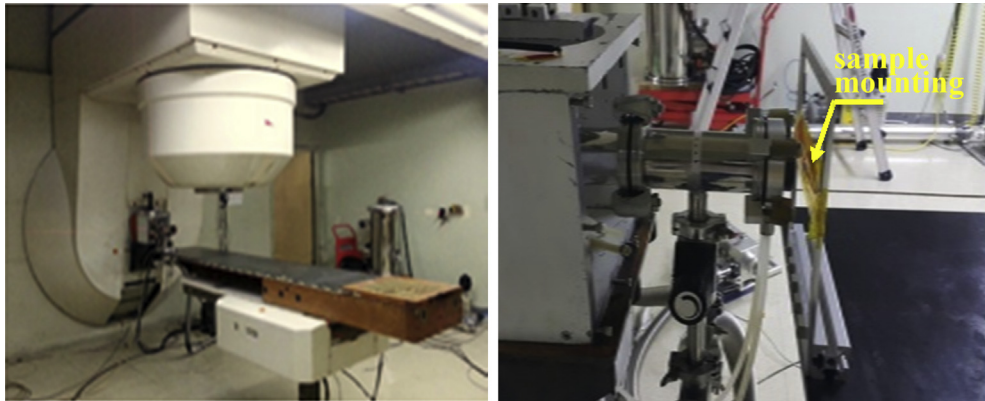
Fig. 2 – MC-50 cyclotron and sample mounting at the end of beam line #2.
