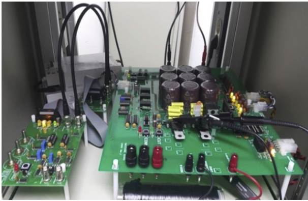
Fig. 5 – Circuit of the system for the turn-off delay time measurement.
