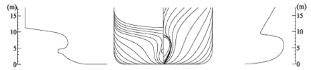
Fig. 4 Body Plan & Side Profile of KCS
