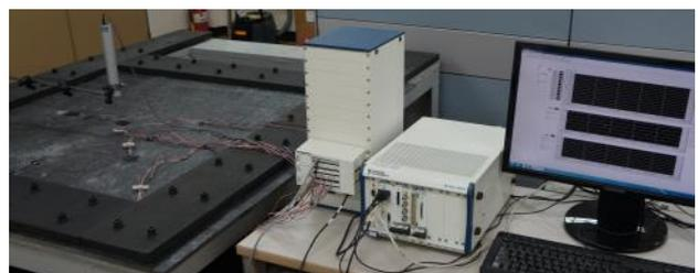
(b) CFRP test panel with DAQ system
