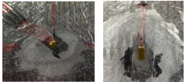
Fig. 8 Installed stacked rosette(left) and uni-axial(right) strain gauges
