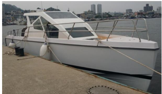
Fig. 1 Picture of CFRP marine leisure boat
