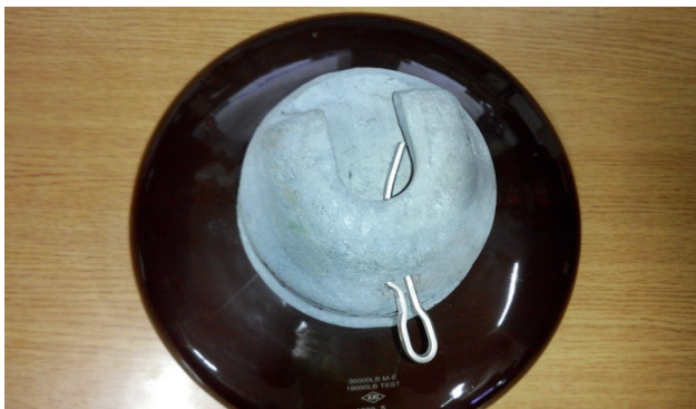
Fig. 1. A suspension-type porcelain insulator used for 154 kV power transmission lines in South Korea by KRI company.
