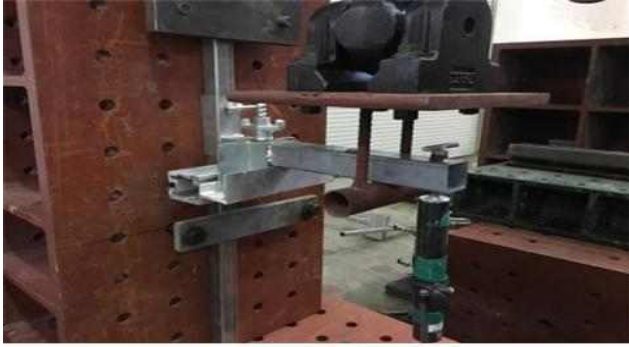
Figure 5. Flexural test of a bracket
