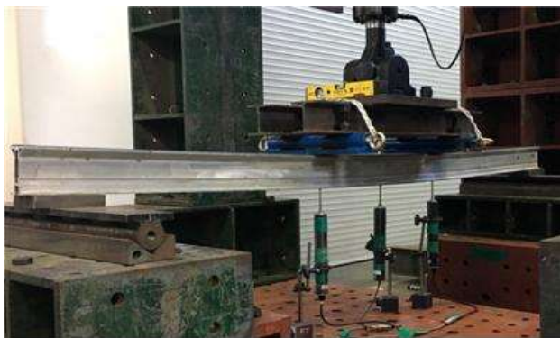
Figure 3. The flexural test of a prop beam
