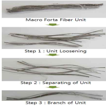
Figure 2. Diffusion step of macro forta fiber
