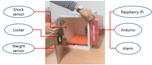
<Figure 8> Prototyped IoT-based Unmanned Home-Delivery Box System
