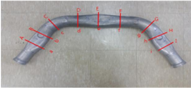
Fig. 4 The thickness measurement of sidemember for hot metal gas forming
