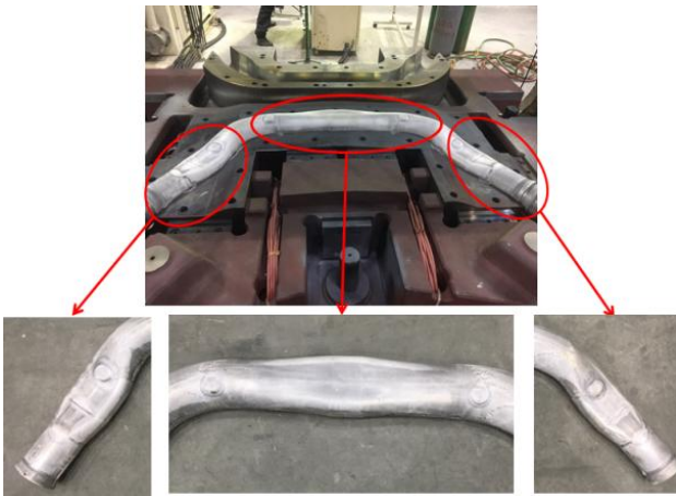
Fig.10 Prototype of sidemember with hot metal gas forming
